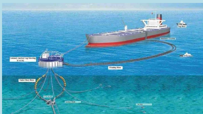
Figure 13: Single Point Mooring (SPM) with Double Pipeline
