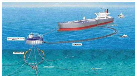
Figure 12: Single Point Mooring (SPM) with Double Pipeline
